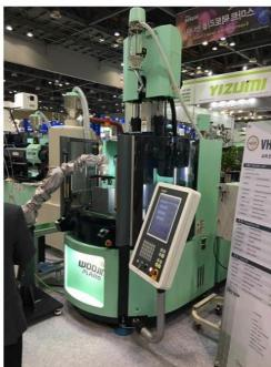
The gamut of injection molding machine scale was on show at Woojin's stand at Koplas, including a 75-tonne vertical press and a 2000tonne two platen unit.
